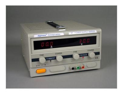
The **digimess**® SM series is a range of general purpose switch mode power supply units featuring high output currents and voltages. All models can operate in either constant voltage or constant current modes and feature large red LED displays for ease of viewing. The switch mode design results in small and light weight units compared to their linear equivalents. All units are supplied with mains leads and operating manuals.
