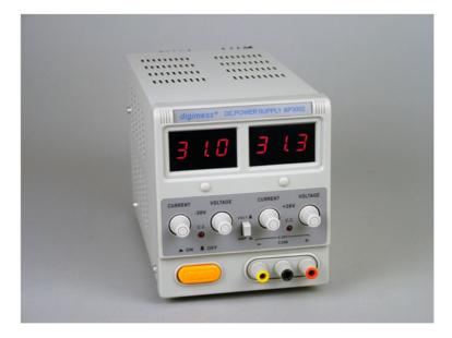
The *digimess*® BP3002 is a low cost general purpose linear dc power supply unit with both plus and minus outputs. The power supply can operate in either constant voltage or constant current modes and features large red LED displays for both voltage and current. Short circuit and current limit protection are included and the BP3002 is supplied with a mains lead and an operating manual.
